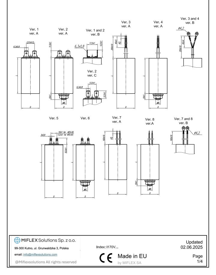
AC METALLIZED POLYPROPYLENE FILM CAPACITORS FOR MOTOR APPLICATIONS IN PLASTIC CASE
